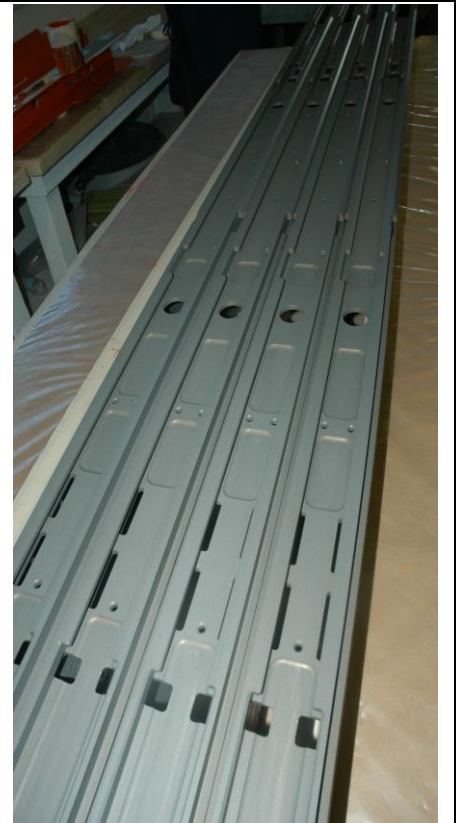
Chem Film/Ano IC (Boric Sulfuric)/Prime/Paint
