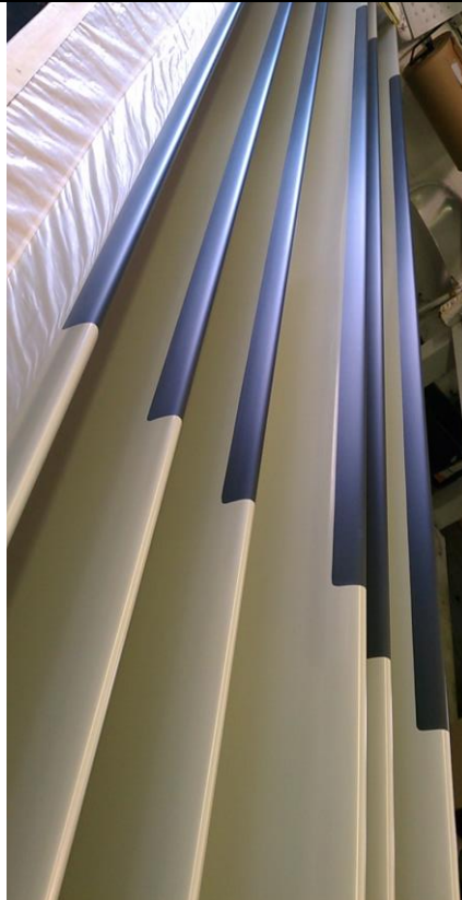
Chem Film/Ano IC (Boric Sulfuric)/Prime/Paint
