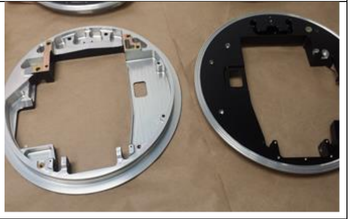
Chem Film/Ano IC (Boric Sulfuric)/Prime/Paint
