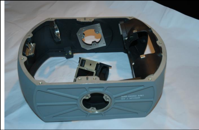
Chem Film (I/3) / Ano (II/Black) / Mask / Brush Nickel Plate / Prime / Paint / Label
